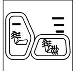
The buttons for the driver's side heated seat are located on the driver's side door panel. The buttons for the passenger's side heated seat are located on the passenger's side door panel.
